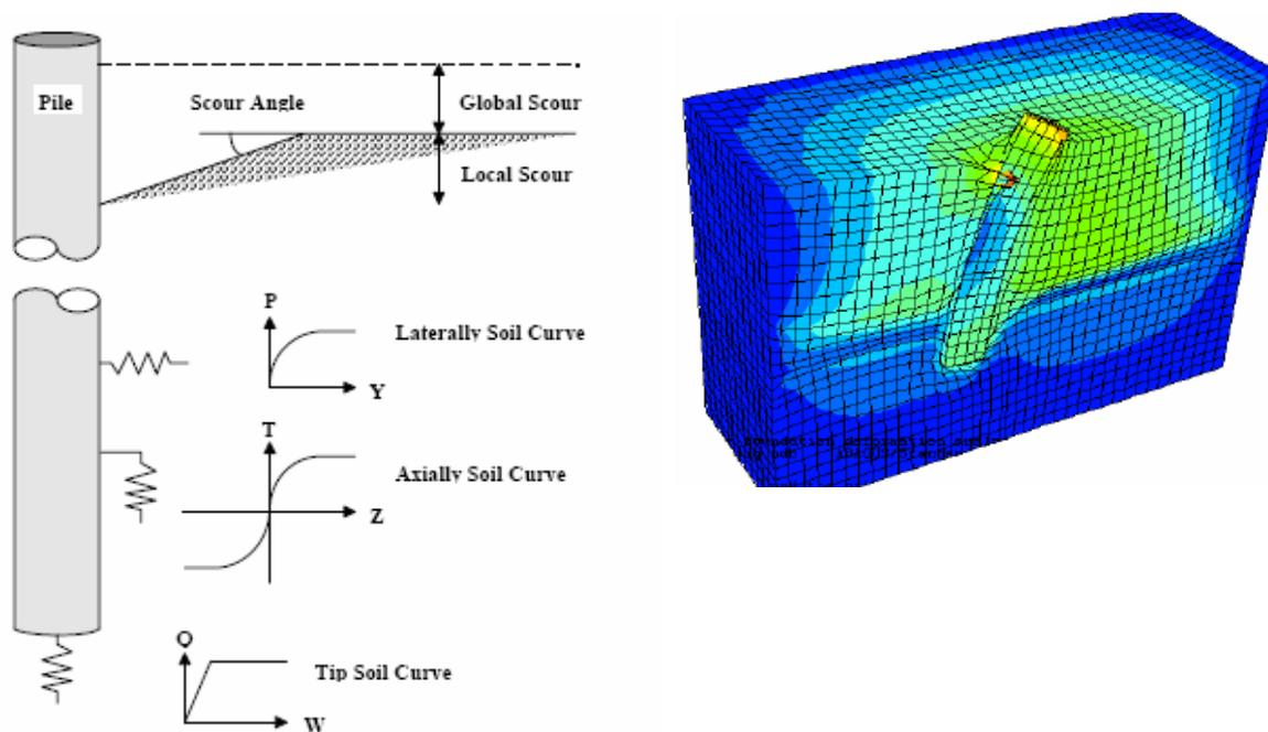
**Figure 2 Modeling the Seabed Pile Interaction and a Typical Simulation Output**
