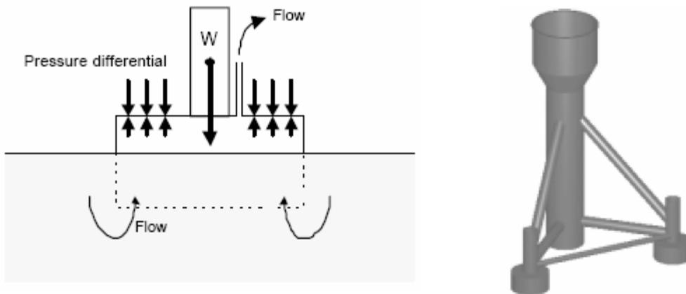
**Figure 3 Suction Cup based Foundation**
