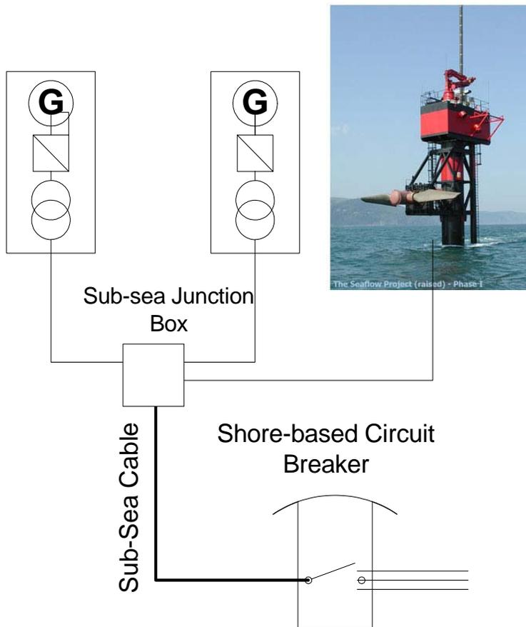
**Figure 5. TISEC System Electrical Interconnection Diagram**
