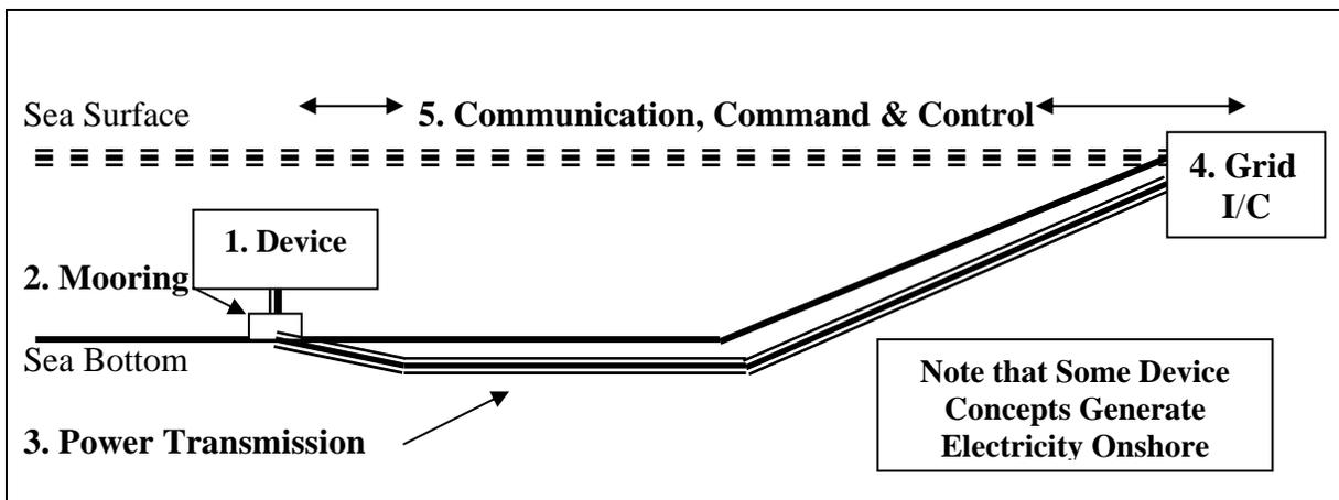
**Figure 1 Tidal In Stream Energy Conversion (TISEC) Power Plant System**
