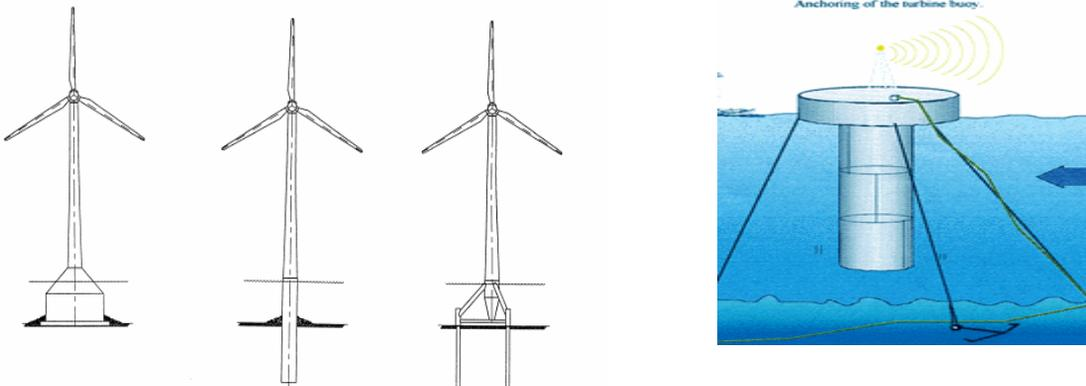
**Figure 1. TISEC Device Foundation Types**
