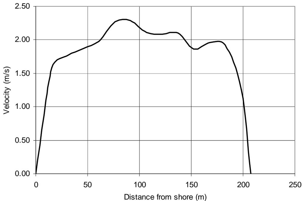
**Figure 6: USGS Measurement Cross Section, velocity at a discharge rate of 63,900 ft<sup>3</sup>/s**
