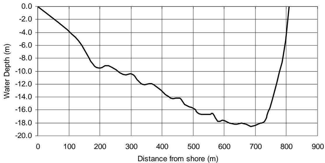
**Figure 50: USGS cross-section showing water at a discharge rate of 219,000ft<sup>3</sup>/s**
