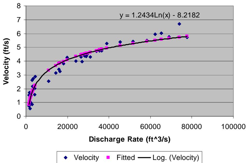
Figure 8: Relationship between velocity and Discharge Rate
