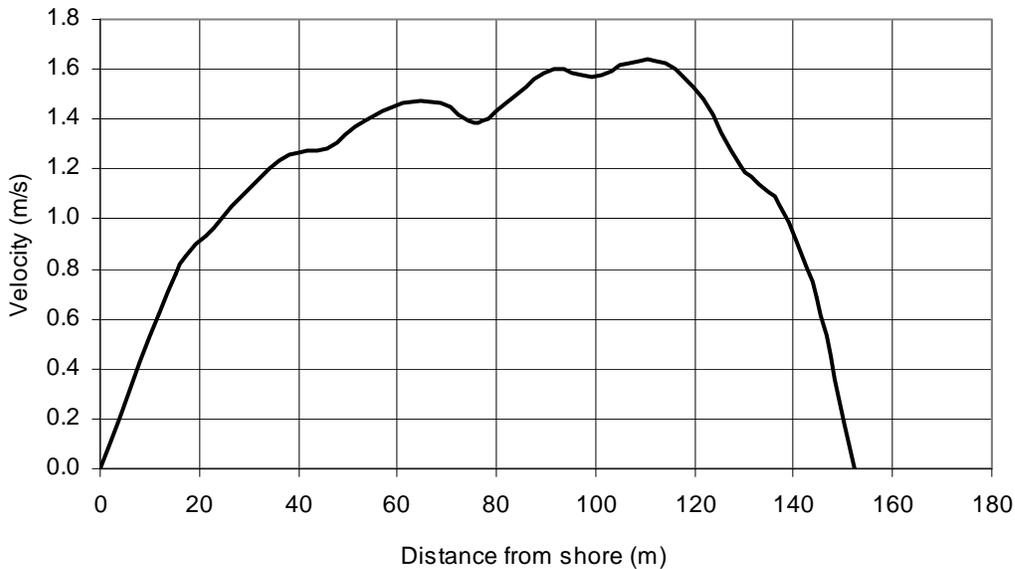
**Figure 60: USGS cross-section showing velocity at a discharge rate of 17,200ft<sup>3</sup>/s**
