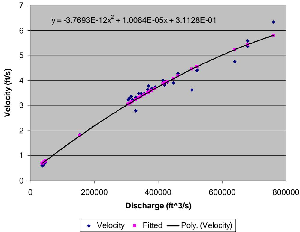
Figure 51: Relationship between Velocity and Discharge Rate
