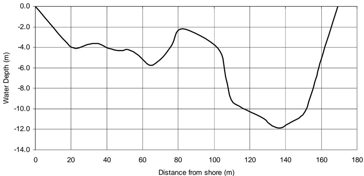
Figure 27: USGS cross-section showing water depth at a discharge rate of 41,200ft<sup>3</sup>/s
