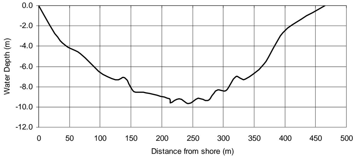
Figure 40: USGS cross-section showing water depth at a discharge rate of 183,000ft<sup>3</sup>/s
