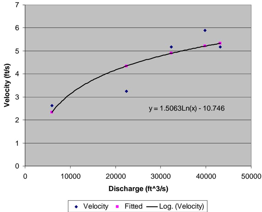
Figure 28: Relationship between Velocity and Discharge Rate
