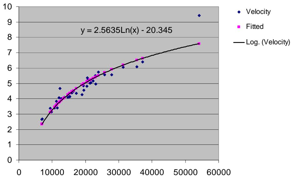
**Figure 62: Relationship between Velocity and Discharge Rate**
