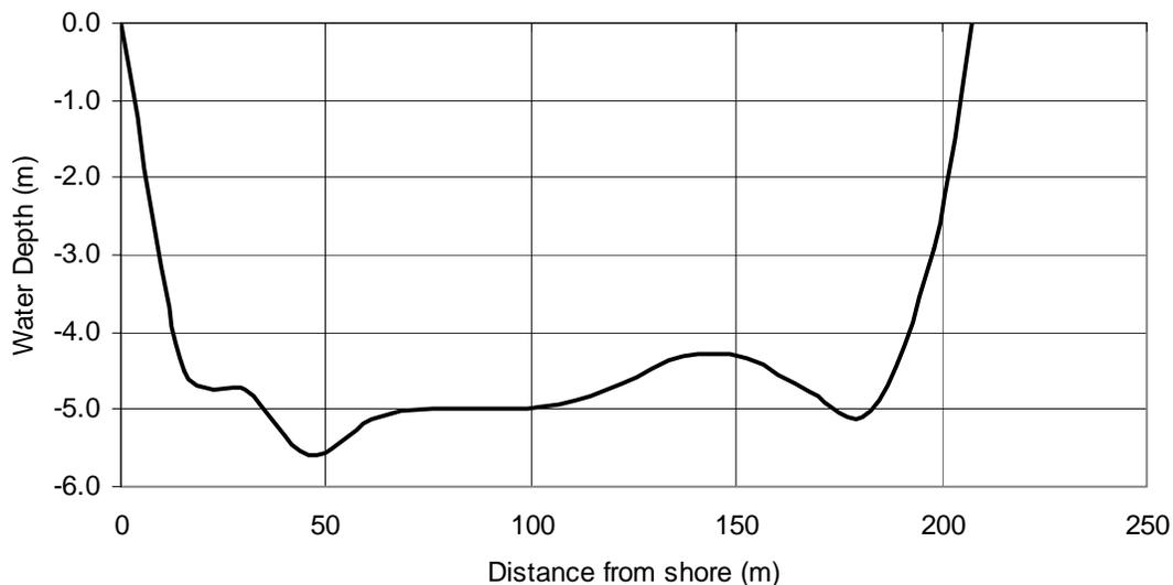
Figure 7: USGS Measurement Cross Section, showing water depth at a discharge rate of 63,900 ft<sup>3</sup>/s
