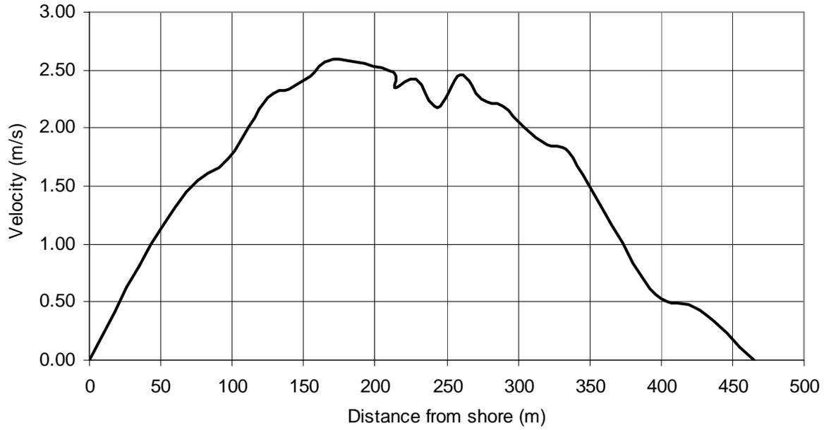
Figure 39: USGS cross-section showing velocity at a discharge rate of 183,000ft<sup>3</sup>/s
