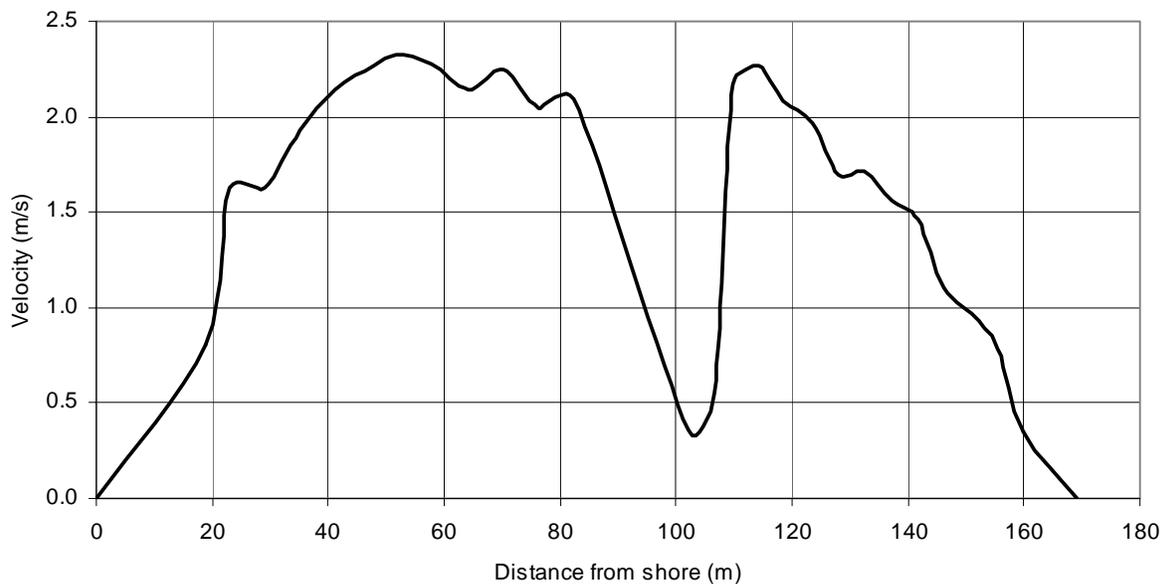
Figure 26: USGS cross-section showing velocity at a discharge rate of 41,200ft<sup>3</sup>/s
