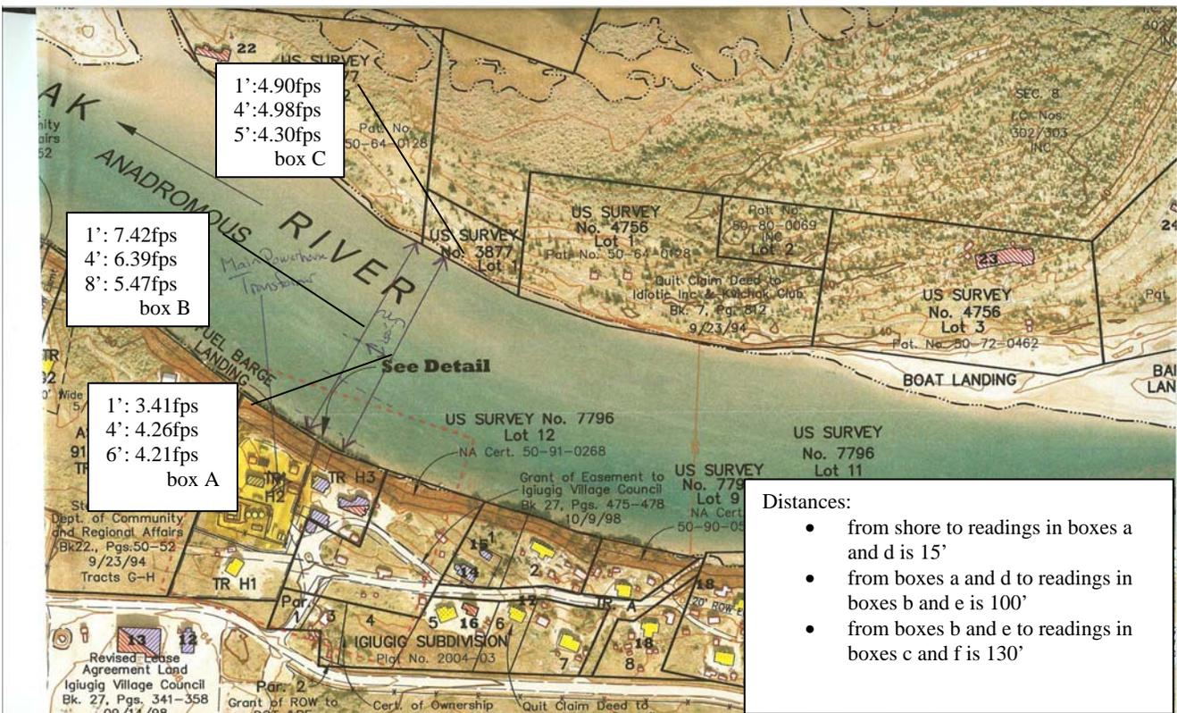
Figure 58: Water velocity readings at proposed site: June 20th 2007
