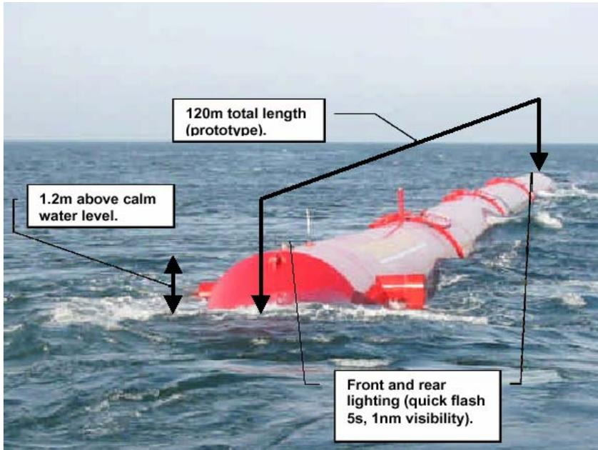
**Figure 5: Pelamis pre-production prototype undergoing sea-trials**
