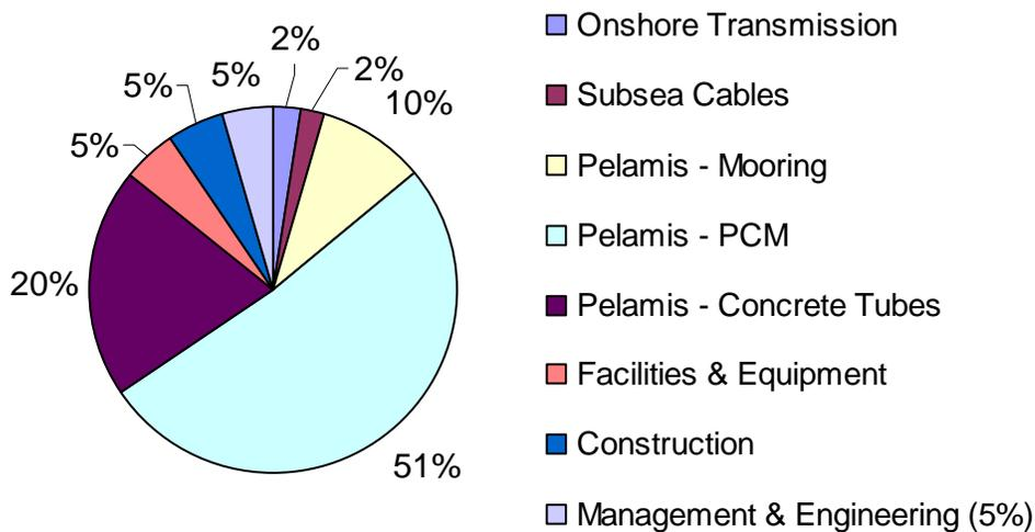
**Figure 21: Installed Cost Breakdown for commercial scale plant**
