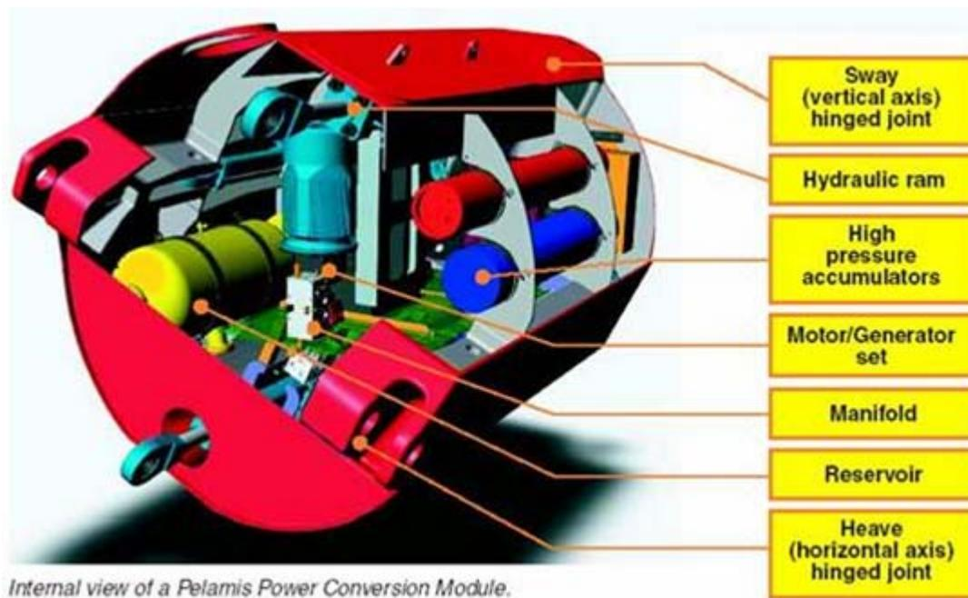
**Figure 8: Internal View of the Pelamis PCM**
