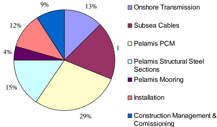
**Figure 19: Pie Chart of cost centers for single unit installation**
