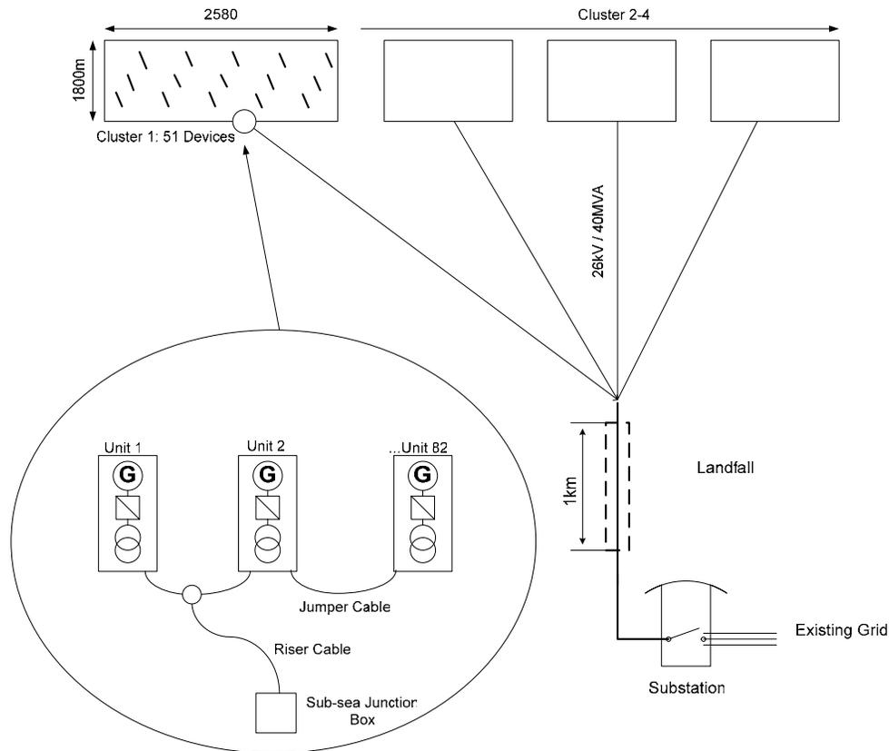
**Figure 17: Overall System Layout and Electrical Connections**
