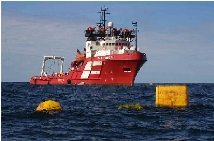
**Figure 14: AHATS class vessel used for prototype installation in UK**
