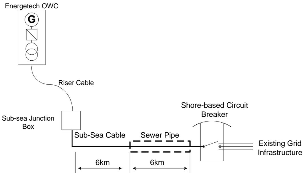
**Figure 12: Electrical Interconnection of a single unit Pilot Plant**
