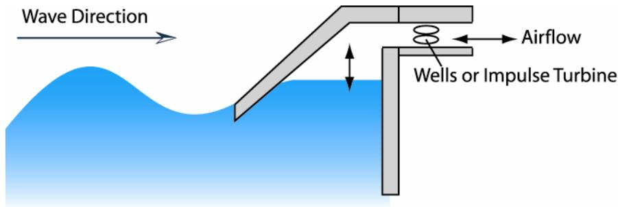
**Figure 6: OWC function principle**
