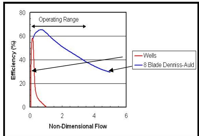
**Figure 9 Turbine variable pitch mechanism (left) Performance comparison (right)**
