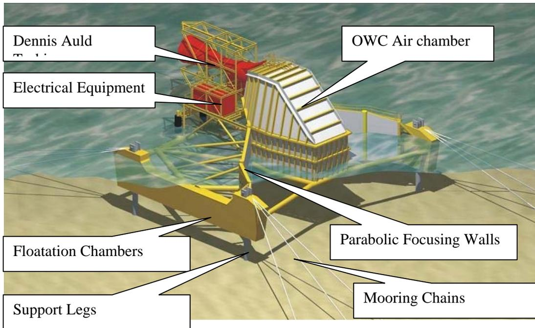
**Figure 7: Energetech's OWC device**
