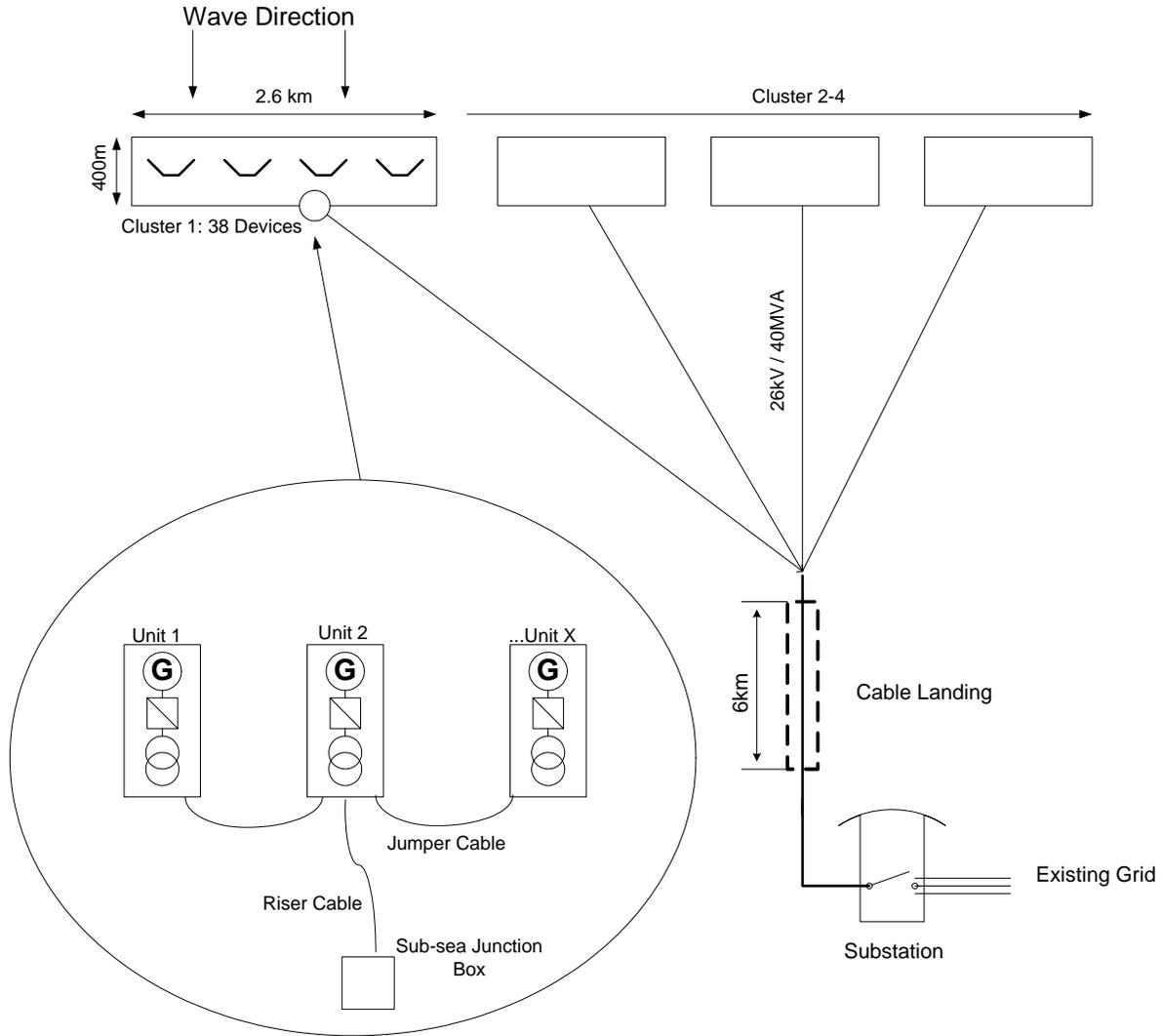
**Figure 13: Overall System Layout and Electrical Connections**
