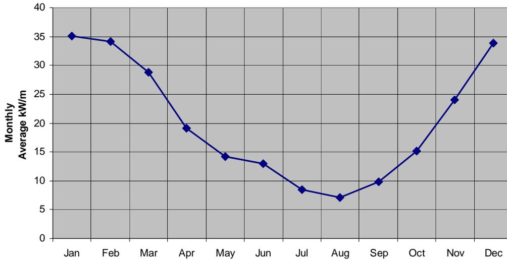
Figure 6: Monthly Average Wave Power Flux at NDBC 46026 (kW/m)
