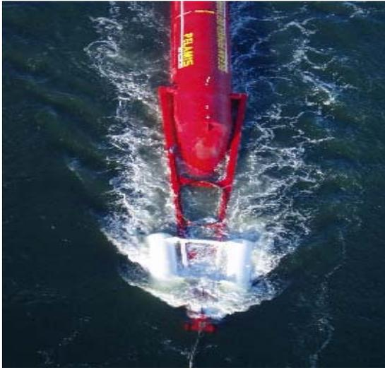
Figure 17: Towing the Pelamis P-750
