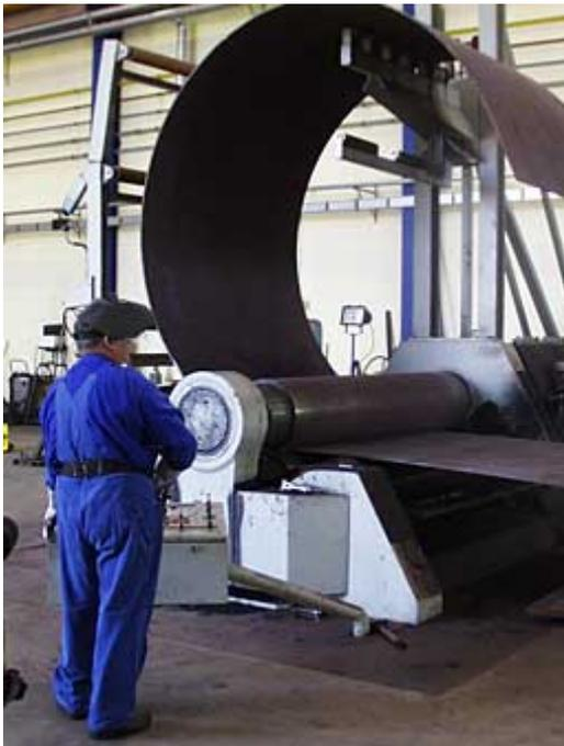
**Figure 11: Manufacturing Steel Tubular Sections**
