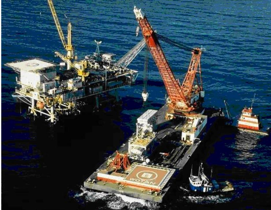
Figure 22 - Manson Construction 600 ton Derrick Barge WOTAN operating offshore
