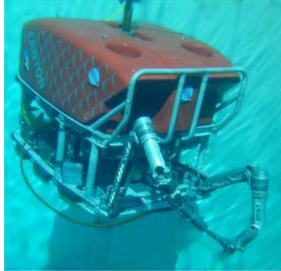
Figure 23 – Two-arm ROV (courtesy of Schilling Robotics [www.ssalliance.com](http://www.ssalliance.com))
