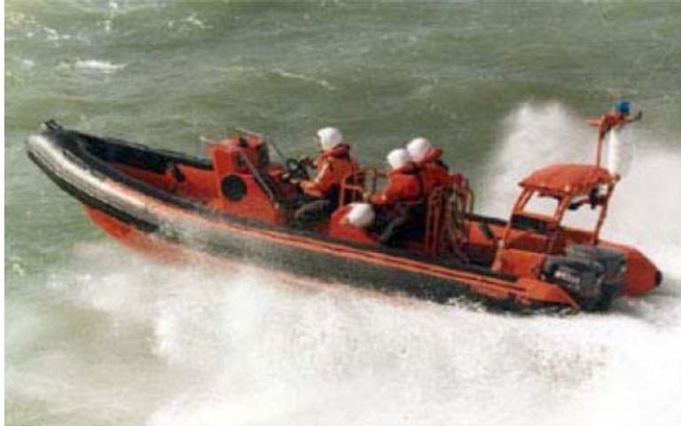
Figure 33 - Typical Rigid Inflatable Boat (RIB)
