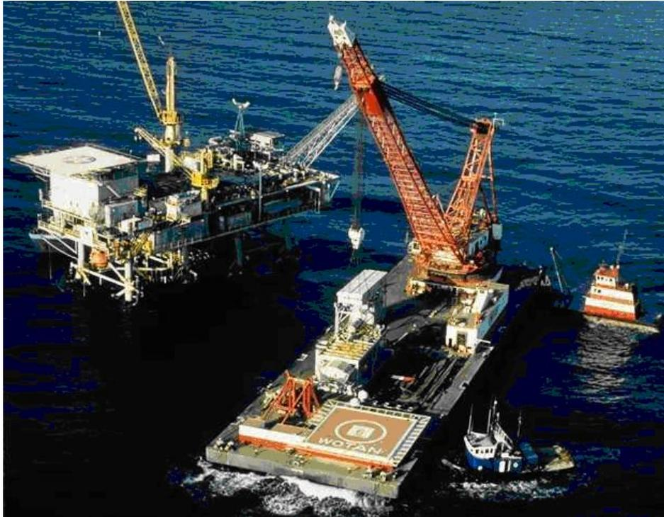
Figure 32 - Manson Construction 600 ton Derrick Barge WOTAN operating offshore (courtesy of Manson Construction)
