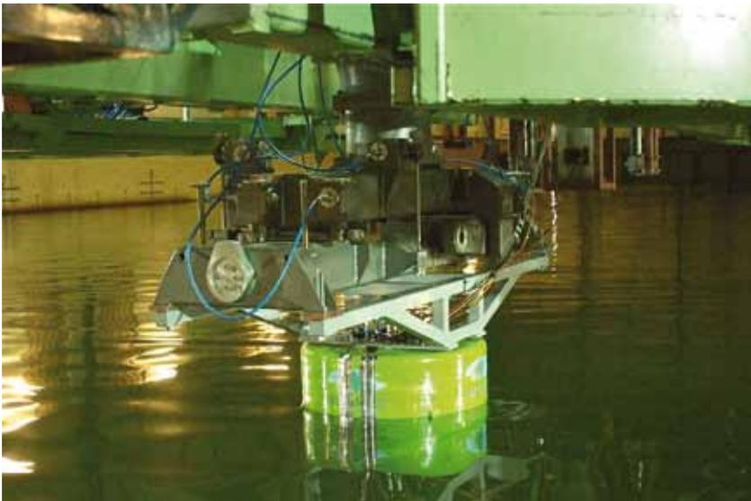
▲ Tank testing of OCEANTEC wave energy device
