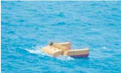
◀ Duck-2 wave energy device under testing
