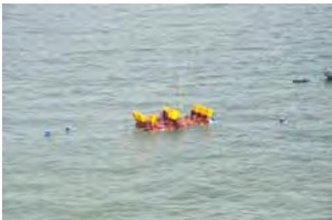
◀ Pendulum wave energy device under testing
