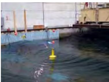
▲ Wave power generation experiment conducted in a wave tank (1/16)
